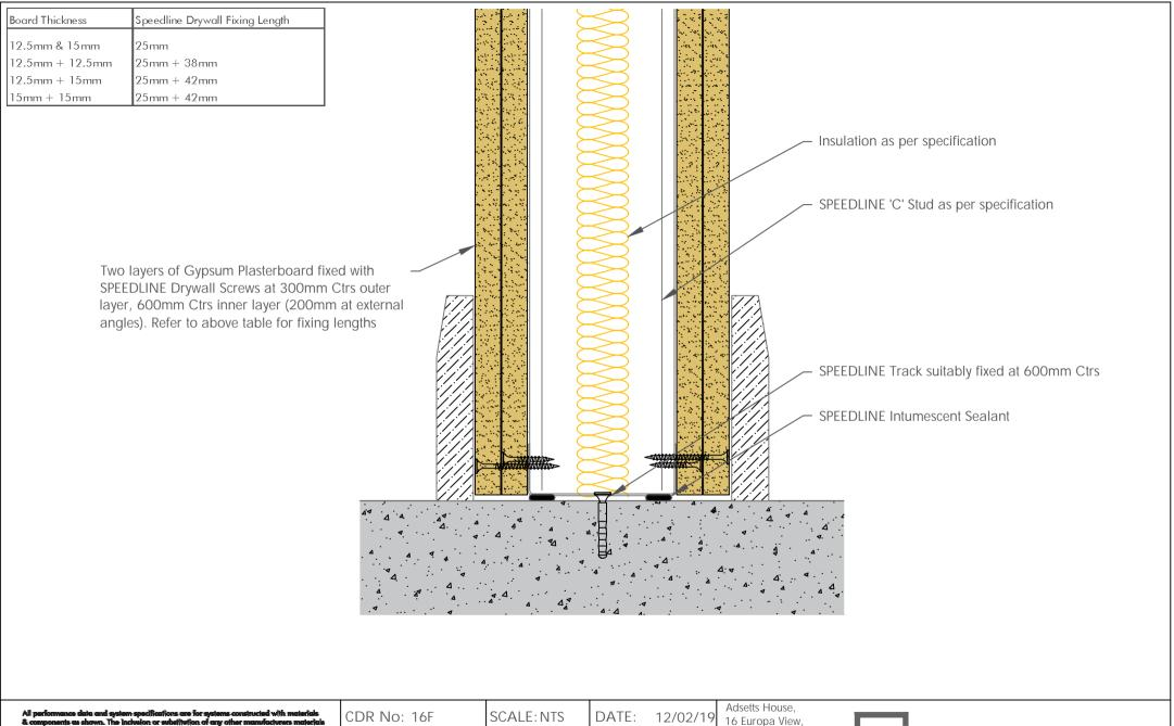
& components as shown. The inclusion or substitution of any other manufacturers materials or components could invalidate test data and system performance and permission must be given in writing by SIG PLC.
